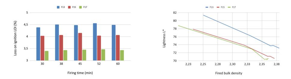
Firing in gas roller kiln at 1200°C with a variable firing cycle.
