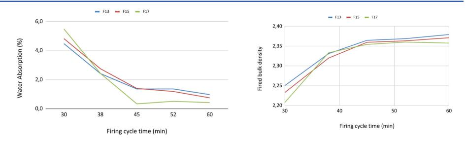
Firing in gas roller kiln at 1200°C with a variable firing cycle.
