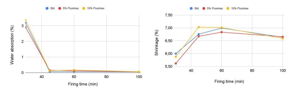
Firing in a roller gas kiln at 1200°C with a variable cycle time.
